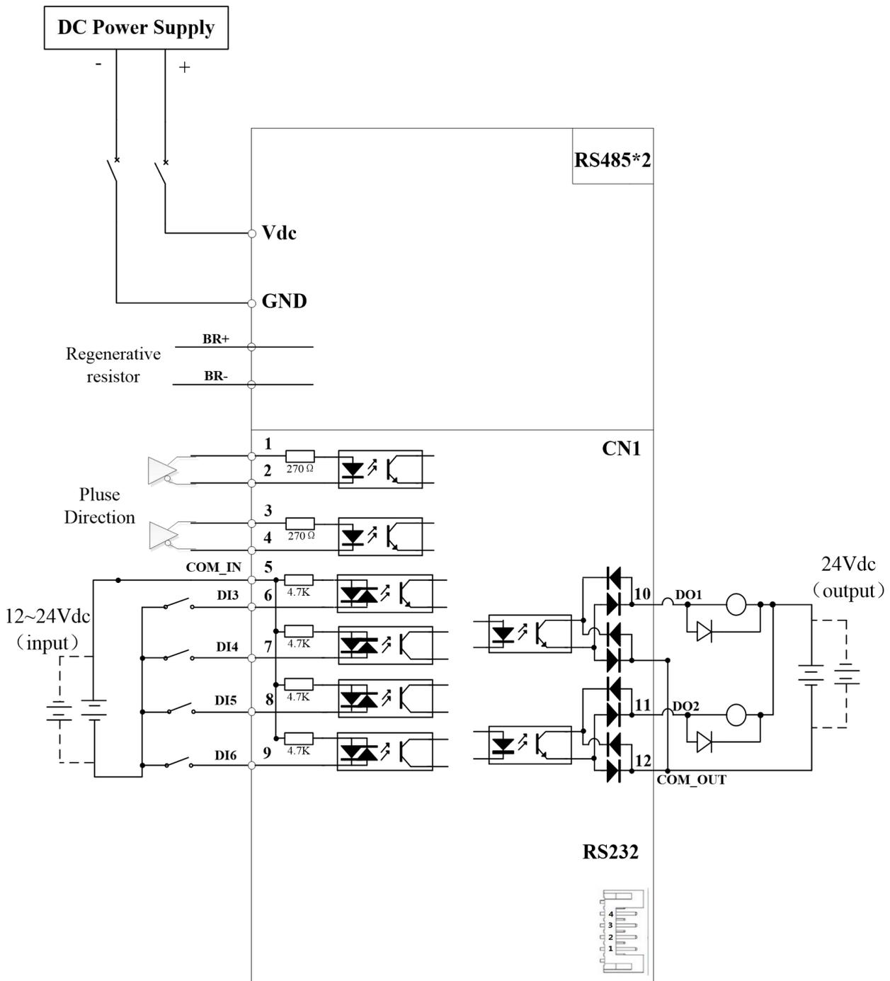
Figure 3.1 Position Control Mode Wiring
