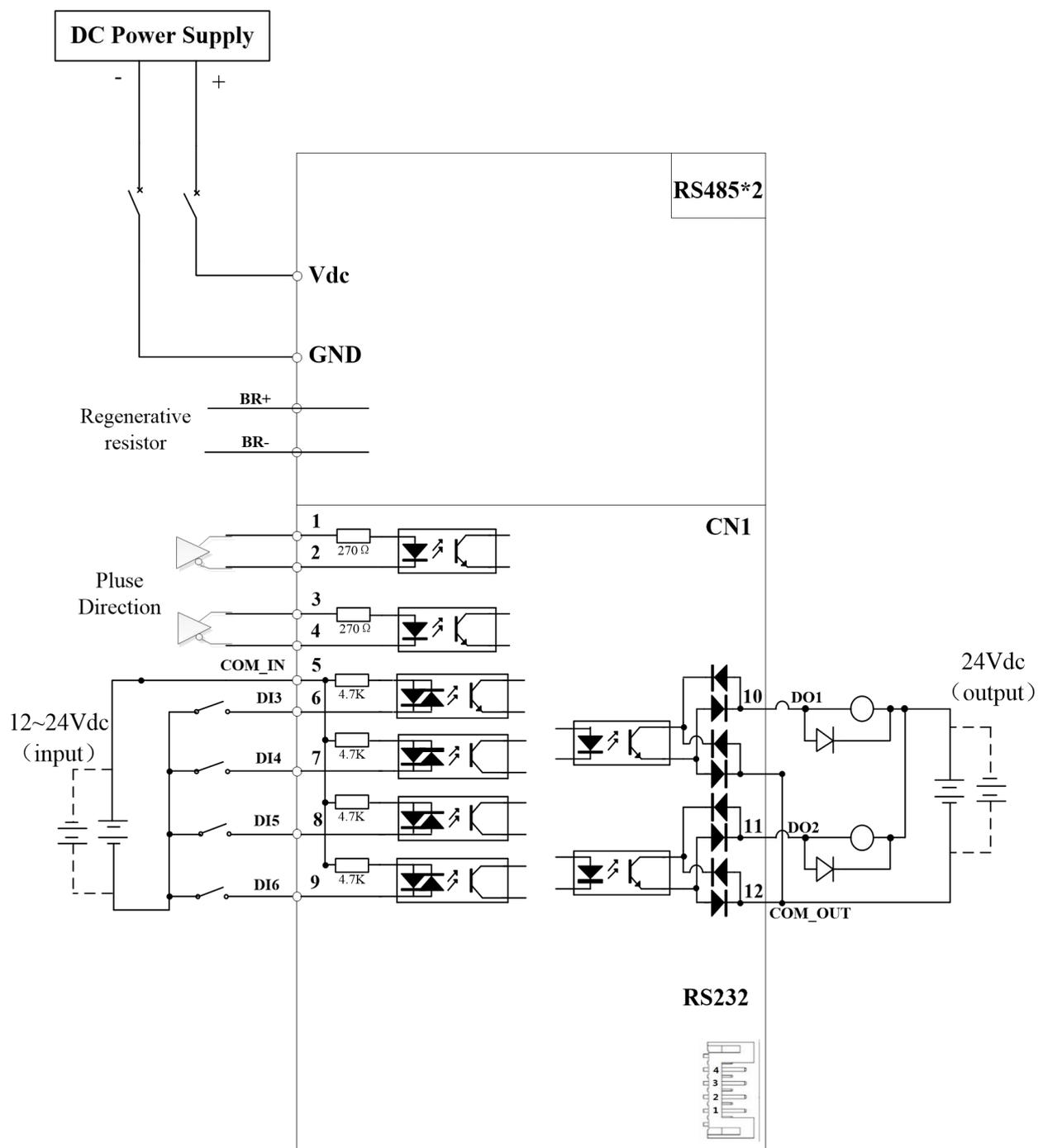
Figure 6-2 Position Mode Wiring
